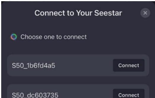
3. If this is the first time your phone or tablet connects to Seestar, the App will remind you to press the reset button on the bottom of the Seestar device to confirm the connection.
